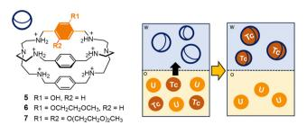
**Fig. 6** Schematized solvent extraction process involving cages **5–7** as extractants: in particular, the cages are employed in the selective back-extraction of Tc (as pertechnetate) from an organic phase containing U in isane.† Successful extraction of Tc was achieved using cages **6–7** as extractants into the aqueous phase (1 mol  $L^{-1}$  HNO<sub>3</sub>).
