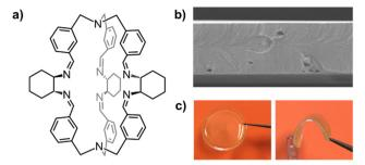
Fig. 13 (a) Schematized structure of a chiral cage employed in the preparation of mechanically robust self-standing membranes with various thickness; (b) SEM image (25 K $\times$ ) of the cross-section of a thin membrane obtained from the neat cage (thickness: 4.3  $\mu$ m); (c) pictures of a  $\sim$ 70  $\mu$ m thick membrane of the same cage (20 mm diameter). Reproduced and adapted with permission from Chem. - Eur. J., 2023, e202301437. 105
