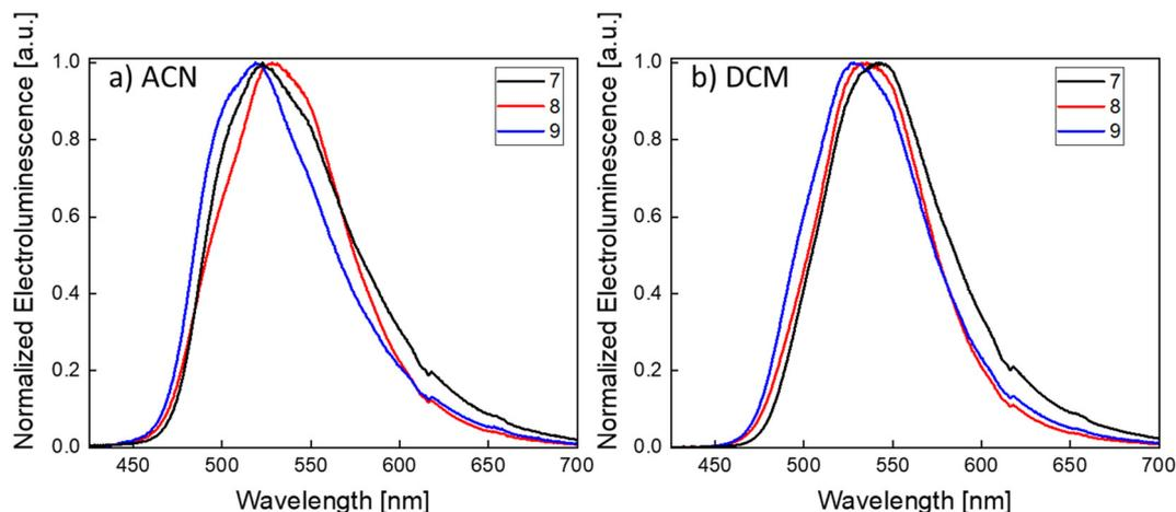
Fig. 6 Normalized electroluminescence spectra of LEC devices ITO/PEDOT:PSS/iTMC:IL(4 : 1)/Al, (iTMC: **7** (black), **8** (red) and **9** (blue)) with the active layer prepared from solutions in ACN (a) and DCM (b).
