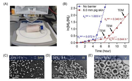
Fig. 7 (A) Experimental setup of photo-RAFT dispersion polymerization under the NIR light ( $\lambda_{max} = 730 \text{ nm}$ ; 60 mW cm<sup>-2</sup>) irradiation passing through 6.0 mm pig skin. (B) Comparison of dispersion photo polymerization kinetics between without barrier and through 6.0 mm pig skin. (C-E) Evolution of morphologies of polymeric nanoparticles synthesized through 6.0 mm pig skin indicated by corresponding TEM images at different time points (t = 7, 9, and 12 hours).
