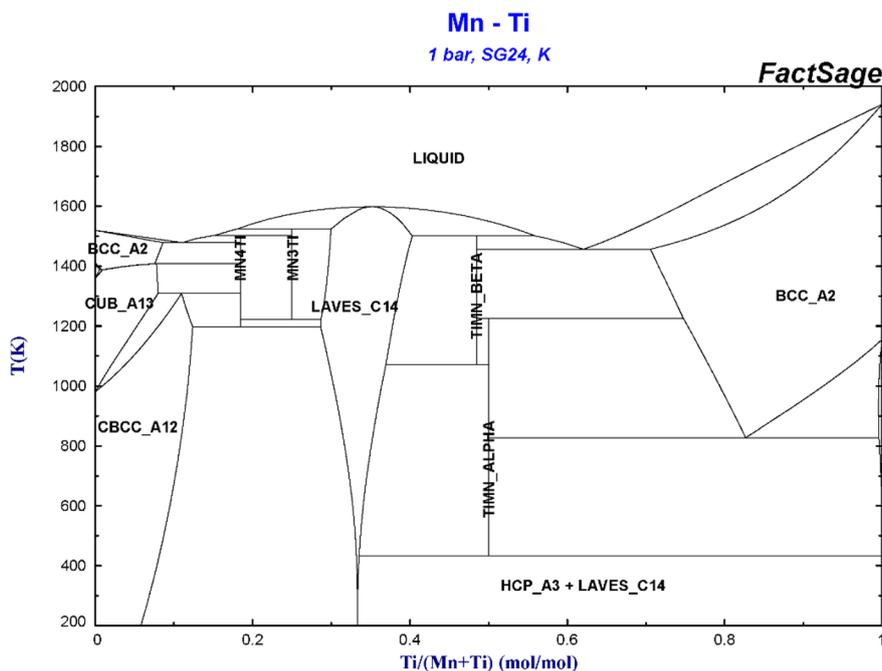
Fig. 2 Binary phase diagram of Mn–Ti.<sup>57,58</sup>
