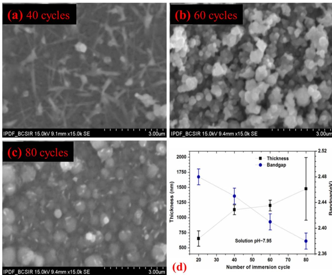
Fig. 9 SEM micrographs of the films grown with different immersion cycles at pH: 7.95 for (a) 40 cycles (b) 60 cycles (c) 80 cycles and (d) film thickness of  $\text{Cu}_2\text{O}$  thin films using different immersion cycles grown by m-SILAR.<sup>37</sup>
