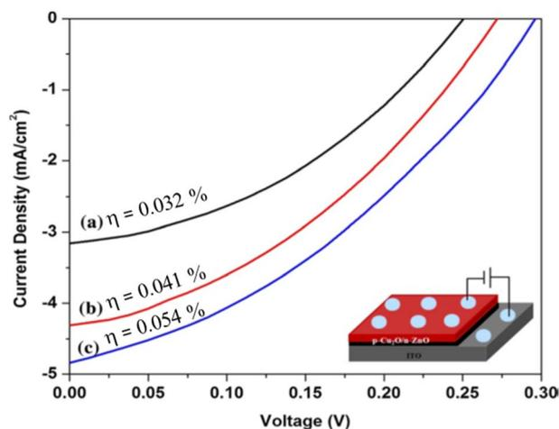
Fig. 11 Current–voltage curve of ITO/ZnO NRs/ $\text{Cu}_2\text{O}$ /Al cells (a) 50 (b) 75 and (c) 100 dip  $\text{Cu}_2\text{O}$  films.<sup>106</sup>
