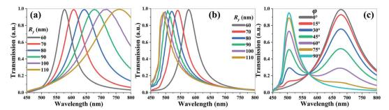
Fig. 4 Transmission spectra of TCF-2 with different  $R_y$  values in (a) TE and (b) TM modes at normal incidence. (c) Transmission spectra of TCF-2 with different  $\varphi$  values from 0° to 90° under the condition of  $R_x = 60$  nm and  $R_y = 90$  nm at normal incidence.
