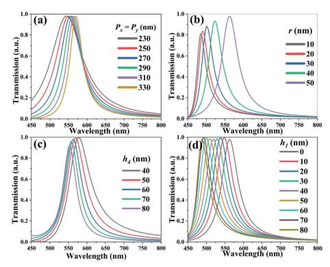
Fig. 2 Transmission spectra of TCF-1 with different values of (a) periods ( $P_x = P_y$ ) from 230 nm to 330 nm, (b) r from 10 nm to 50 nm, (c) thickness of Ag nanoholes ( $h_3$ ) from 40 nm to 80 nm, and (d)  $h_1$  from 0 nm to 80 nm under normal TE-polarized incident light.
