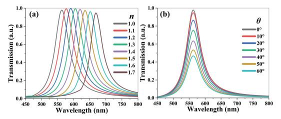
Fig. 3 Transmission spectra of TCF-1 (a) exposed to the ambient environment with different n values from 1.0 to 1.7 under normal TE-polarized incident light and (b) with different  $\theta$  values from 0° to 60° in TE mode.
