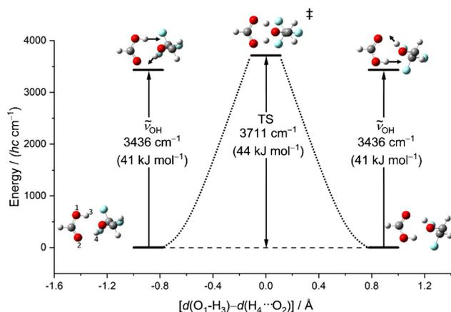
Fig. 6 Energy profile calculated at B3LYP-D3(BJ)/def2QZVP level (ZPE corrected) for the proton exchange promoted by the symmetric OH stretch vibration in the most stable  $(T_g^g F)$  dimer. As the exchange coordinate, the difference between the chemical and the hydrogen-bonded distances of the two jumping protons from the acid oxygens is chosen. The transition state ( $1620i\text{ cm}^{-1}$ ), where this difference vanishes, has  $C_s$  symmetry.
