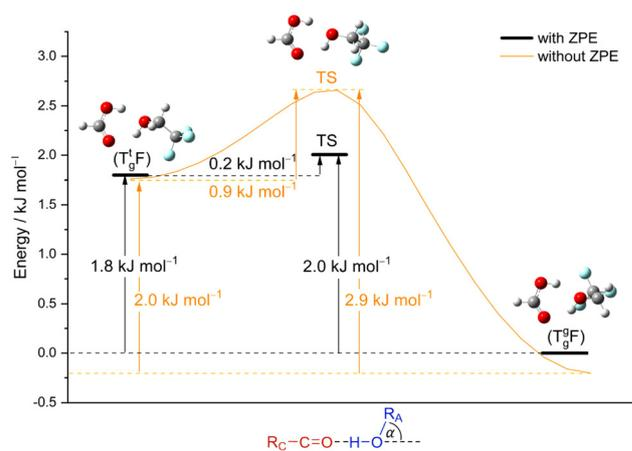
Fig. 5 Energy profile calculated at B3LYP-D3(BJ)/def2QZVP level for the isomerism of the metastable  $(T_g^g F)$  complex on the left to the global minimum  $(T_g^t F)$  structure on the right (lone pair switch) along the hinge angle. Shown with and without zero-point vibrational energy.
