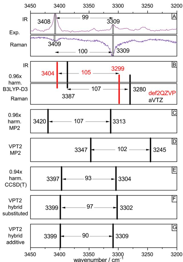
Fig. 4 Comparison of experimental OH stretching band positions (from Fig. 2, trace c, IR and Fig. 3, trace c, Raman) and their splitting with harmonic and anharmonic predictions for the  $(T_g^g F)$  dimer. See text for explanations.
