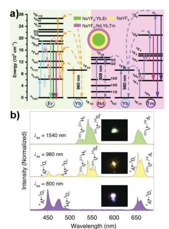
Fig. 2 (a) Proposed multiple excited state absorption and energy transfer mechanism in Nd<sup>3+</sup>, Yb<sup>3+</sup>, Er<sup>3+</sup>, and Tm<sup>3+</sup>-codoped UCNC.<sup>76</sup> (b) Upconversion emission spectra of UCNCs shown in (a) and the corresponding photo of UCNC films excited using  $\lambda_{ex}$  = 800, 980 and 1540 nm laser excitation.<sup>76</sup> Reprinted with permission from ref. 76. Copyright 2020, Nature Publishing Group.
