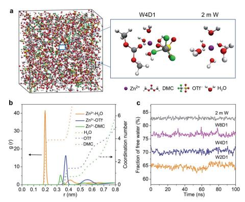
Fig. 2 MD studies of the  $Zn^{2+}$  solvation structure. (a) Snapshot of the MD simulation cell for the W4D1 electrolyte, and the representative  $Zn^{2+}$  solvation structures in W4D1 and 2 m W electrolytes. (b) RDFs of Zn-O (H<sub>2</sub>O), Zn-O (DMC) and Zn-O (OTf<sup>-</sup>) pairs, and the coordination number in the W4D1 electrolyte. (c) Fraction of free water (not solvating to  $Zn^{2+}$ ) in the H<sub>2</sub>O + DMC electrolytes with a 100 ns simulation time.
