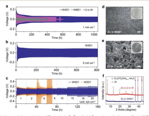
Fig. 4 Electrochemical test and characterization of Zn anodes in Zn/Zn cells. (a) Comparison of voltage profiles in W4D1, W8D1 and 2 m W electrolytes at 1 mA cm $^{-2}$ . (b) Cycling performance in the W4D1 electrolyte at 5 mA cm $^{-2}$ . (c) Rate capability of Zn/Zn cells with W4D1 and W2D1. (d, e) SEM images (scale bar, 10  $\mu$ m) and (f) XRD patterns of Zn anodes after 300 cycles. Insets of (d, e) show the optical images of cycled Zn anodes.
