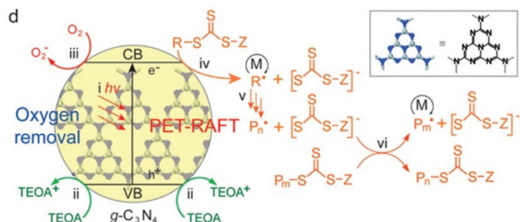
Fig. 13 Proposed mechanism of PET-RAFT polymerization using g-C 3 N 4 as the photocatalyst in the presence of TEOA. Reproduced from ref. 36 with permission from the American Chemical Society, copyright 2017.
