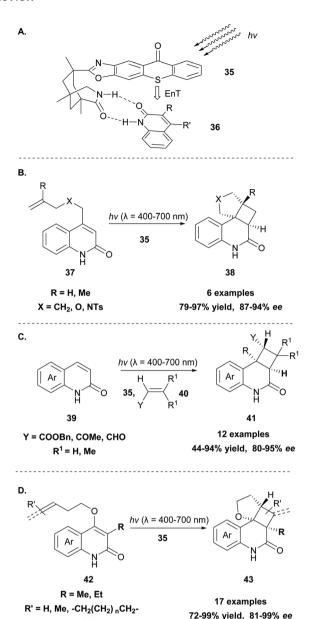
Scheme 10 (A) Hydrogen bond complex formation between chiral thioxanthone 35 and general lactam substrate 36 and (B-D) enantioselective [2+2] photocycloadditions in the presence of chiral sensitizer 35.
