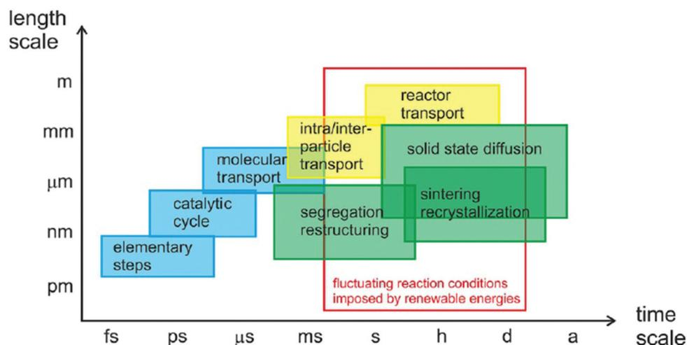
Fig. 3 Time scale of various processes in catalytic reactions. All panels reproduced with permission.<sup>29</sup> Copyright 2017, John Wiley and Sons.
