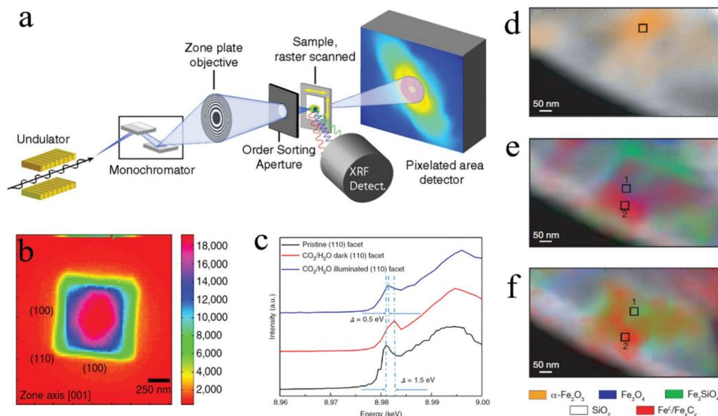
**Fig. 7** (a) STXM and SXFM setup; Copyright 2014, National Academy of Sciences; (b) SXFM image of a  $\text{Cu}_2\text{O}$  nanoparticle; (c) scanning X-ray nanospectroscopy of the (110) facet; Copyright 2019, Springer Nature; (d) to (f) chemical contour images of the catalyst under different treatments; Copyright 2008, Springer Nature. All panels reproduced with permission.<sup>148,156,160</sup>
