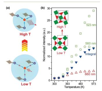
Fig. 7 (a) Thermal promotion of energy delivery to activator ions by lattice contraction in negative thermal expansion crystals. (b) Normalized emission intensities of  $Yb_2W_3O_{12}$ :Er (6%) nanocrystals as a function of temperature. Inset: schematic of the lattice contraction and distortion as the temperature increases. Adapted with permission from ref. 101. Copyright 2019, Wiley-VCH.
