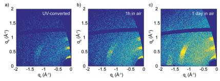
Fig. 4 Evolution of the GIWAXS patterns for the (PEA)<sub>2</sub>CuCl<sub>4</sub> film in air (a) just after irradiation with UV light, (b) 1 hour after irradiation and (c) 1 day after irradiation. The incident angle was 0.2°. Note that the sample was kept in the same place during this measurement, to ensure that a quantitative comparison between the different images can be made
