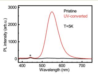
Fig. 6 Photoluminescence spectra for pristine (black line) and UV-converted (red line) (PEA)<sub>2</sub>CuCl<sub>4</sub> films acquired at 5 K. The peak that is marked with an asterisk is a measurement artifact due to stray background light.
