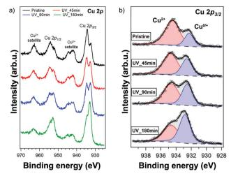
Fig. 5 (a) XPS spectra of the Cu 2p core level region of a pristine (PEA)<sub>2-</sub> CuCl<sub>4</sub> film and after exposing it to UV light for various durations. The film was UV-converted in situ; XPS spectra were recorded after 45, 90 and 180 minutes. (b) Fits of the high-resolution Cu 2p<sub>3/2</sub> peaks with Cu<sup>2+</sup> (red curve) and Cu<sup>0/+</sup> (blue curve) signals for the different data depicted in (a).
