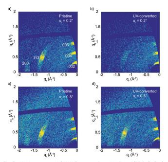
Fig. 3 Wedge corrected GIWAXS patterns for a thin film of (PEA)<sub>2</sub>CuCl<sub>4</sub> (a and c) before and (b and d) after UV irradiation measured at two different incident angles ( $\alpha_i = 0.2^{\circ}$  ( $\sim 25$  nm) for a and b and  $\alpha_i = 0.8^{\circ}$  ( $\sim 2$   $\mu$ m) for c and d).
