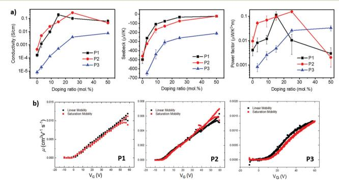
Fig. 4 (a) Thermoelectric properties of doped polymers at different doping concentrations including electrical conductivities, Seebeck coefficients and power factors. (b) Transistor properties of pristine P1, P2 and P3.
