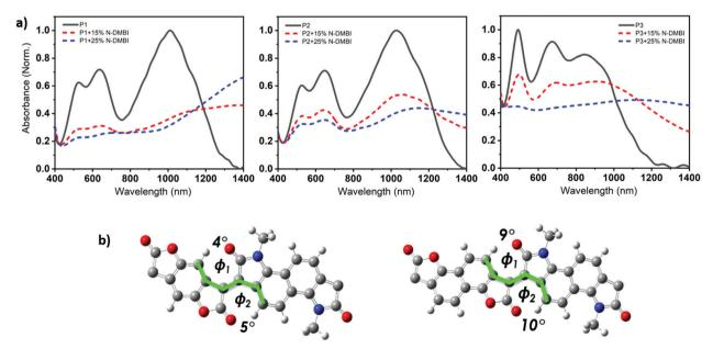
Fig. 3 (a) UV-Vis-NIR absorption spectra of the pristine and doped (at 15 and 25 mol% N-DMBI doping ratio) thin films of P1, P2, and P3. (b) DFToptimized molecular model of the phenyl-bis-lactone and naphthalene-bis-lactone fragments (ωB97XD/6-31G\*\*)
