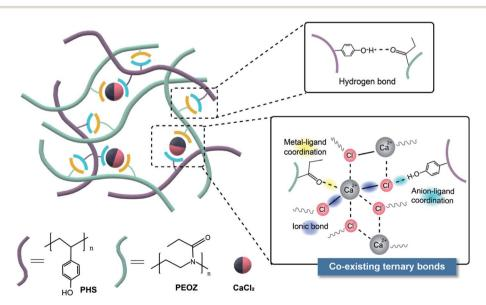
Scheme 1 Schematic diagram of the self-healing structure composed of the hydrogen bonds, metal-ligand coordination, and ionic bonds.
