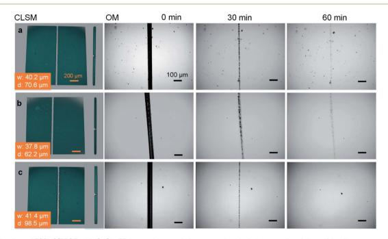
Fig. 1 Self-healing of 30PHS/PEOZ with CaCl<sub>2</sub>. 3D laser microscopic images and optical photographs of the self-healing process of (a) 30PHS/ PEOZ, 30PHS/PEOZ with (b) 0.17 equivalent CaCl<sub>2</sub> and (c) 0.25 equivalent of CaCl<sub>2</sub>. The healing rate of 30PHS/PEOZ was improved by the addition of 0.25 equivalent of CaCl<sub>2</sub>. CLSM: confocal laser scanning microscope, OM: optical microscope, w: width, d: depth.
