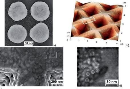
Fig. 2 (a) SEM image of a fragment of the Au nanodisk array (four large bright spots) covered with CdSe NCs (small bright spots). (b) AFM image of a Klarite® structure with a submonolayer coverage of CdSe NCs. CdSe NCs are not clearly resolved in the image. The white rectangle indicates the area shown in the SEM image in (c). (d) A fragment of the SEM image, marked by the white rectangular in (c), showing submonolayer coverage of the surface by CdSe NCs.
