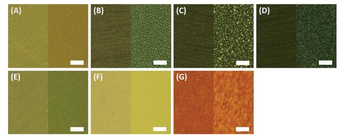
Fig. 2 Optical images (250x) of surfaces of: (A) unfilled epoxy, (B) epoxy-carbon black composite, (C) epoxy-graphene composite, (D) epoxy-MWCNT composite, (E) epoxy-SiO<sub>2</sub> composite, (F) unfilled polypropylene, (G) PP-Fe<sub>2</sub>O<sub>3</sub>. The left half of each image shows un-weathered sample and the right half shows samples weathered for 2500 h in an accelerated wet weathering chamber. Scale bar is 250 µm for all images.
