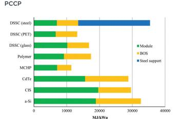
**Fig. 3** Cumulative energy demand for the production of a virtual 3 kW h solar harvesting rooftop photovoltaic installation for various thin-film technologies. Reproduced with permission from Elsevier.<sup>7</sup>
