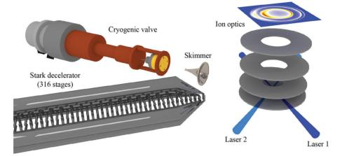
Fig. 1 Schematic representation of a crossed beam apparatus. A beam of NO radicals is passed through a Stark decelerator and scattered with a pulsed beam of para-H2 or ortho-D2. The inelastically scattered NO radicals are state-selectively ionised using two pulsed lasers and detected using velocity map imaging. Only the last section of the Stark decelerator is shown. Reprinted with permission from Gao et al.,58 copyright 2017 American Chemical Society.
