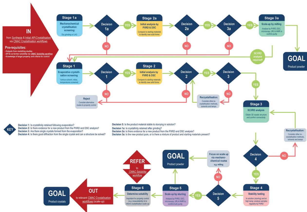
Fig. 1 CMAC multicomponent (MC) material screening workflow. The workflow is driven by the decision points as indicated in the text; these capture the key elements indicating if the co-crystallisation process is likely to have value. Light blue squares indicate points at which the CCDC software tools are implemented. Decision 1: is crystallinity retained following evaporation?; Decision 2: is there evidence for a new product from the PXRD and DSC analysis?; Decision 3: are there single crystals formed from the evaporation?; Decision 4: is there good diffraction from the single crystal and can a structure be solved?; Decision 5: is the product material stable to slurrying in solution?; Decision 1a: is crystallinity retained after grinding?; Decision 2a: is there evidence for a new product from the PXRD and DSC analysis?; Decision 3a: is the new product pure, or is there a mixture of product and starting materials present?
