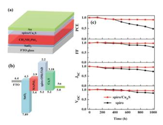
Fig. 14 (a) Schematic illustration of the device structure of a planar n-i-p MAPbl<sub>3</sub> solar cell, with the spiro-OMeTAD/Cu<sub>x</sub>S bilayer; (b) energy band diagram of the PSC; (c) PCE, FF,  $J_{\rm SC}$ , and  $V_{\rm OC}$  as a function of ambient storage time of devices with different HTLs. 114
