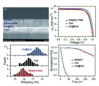
Fig. 12 (a) Cross-sectional SEM image of an inverted PSC with Cu@Cul as the HTM and PCBM as the ETM; (b) best J-V data; (c) histograms of cell efficiencies among 30 cells of PSCs with various HTMs; and (d) stability of PSCs with PCBM as the ETM and various HTMs stored in air at RT with a humidity of about  $45\%.^{108}$
