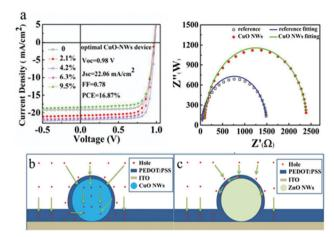
Fig. 20 (a) J-V curves of PSCs with different coverage of CuO NWs, under 100 mW cm<sup>-2</sup> illumination (AM 1.5G) and Nyquist plots of PSCs without and with the optimal coverage of CuO-NWs in the dark and (b) schematic illustration of hole transport with CuO NWs. 129
