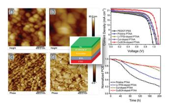
Fig. 10 AFM height and phase images of the perovskite films on different PTAA layers: (a and c) pristine, (b and d) CuSCN-doped cases; (right) J-Vcurves of the PSCs based on pristine and doped PTAA as HTLs (up) and normalized PCE (down) of the PSCs based on pristine and doped PTAA for 200 h. (central image) Device architecture<sup>98</sup> (reprinted (adapted) with permission from ACS Appl. Energy Mater., 2019, 23, 1932-1942, Copyright 2019 American Chemical Society)
