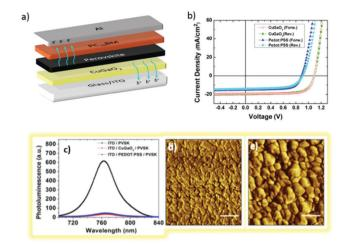
Fig. 23 (a) The structure of p-i-n PSCs (ITO/CuGaO<sub>2</sub>-NPs/CH<sub>3</sub>NH<sub>3</sub>PbI<sub>3</sub>/  $PC_{70}BM/Al)$ ; (b) J-V curves under 1 sun illumination; (c) photoluminescence spectra of CH3NH3Pbl3 on top of ITO, ITO/CuGaO2-NPs, and ITO/PEDOT:PSS electrodes; (d) AFM images of ITO/CuGaO2 and (e) ITO/CuGaO2/CH3NH3Pbl3 films (scale bar = 500 nm). <sup>137</sup>
