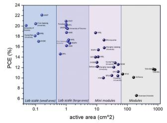
PCEs for lab-scale and large area cells and modules
