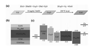
Fig. 21 (a) Preparation process of Cu<sub>2</sub>O and CuO films; (b) device structure; and (c) energy level diagram. 130
