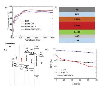
Fig. 7 (a) Transmittance spectra of ITO, ITO/r-GO, ITO/CuSCN, ITO/ r-GO/CuSCN; (b) schematic diagram of the fabricated PSC; (c) energy level diagram of the fabricated PSC; and (d) light soaking stability of the unsealed PSCs fabricated by r-GO, CuSCN and r-GO/CuSCN HTLs.93
