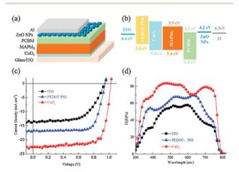
Fig. 22 (a) Schematic of the CuO<sub>x</sub>/ZnO based device structure; (b) energylevel diagram of the corresponding device; (c) J-V curves and (d) EQE spectra of the PVSCs without or with different HTLs. 135
