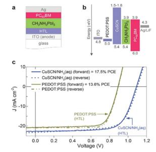
Fig. 6 (a) Schematic cross-section of the cell architecture employed; (b) corresponding material energetics; and (c) J-V characteristics measured under simulated 1 sun solar illumination for the champion CH<sub>3</sub>NH<sub>3</sub>PbI<sub>3</sub> solar cells based on CuSCN/NH<sub>3</sub> (aq) and PEDOT:PSS HTLs.90
