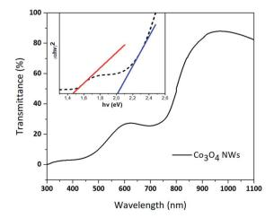
Fig. 4 Transmittance spectra of the  $\text{Co}_3\text{O}_4$  NRs grown on glass substrate, 400 nm long. (Inset) Band gap measurement of  $\text{Co}_3\text{O}_4$  nanorods using Tauc plot method.
