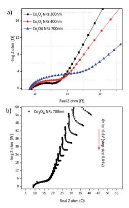
Fig. 8 (a) Nyquist plots of  $Co_3O_4$  electrodes (-Z'' vs. Z') recorded after 10 ion diffusion cycles. (b) Series of impedance plots with different polarization potential ranging from -0.6 to 0 V.
