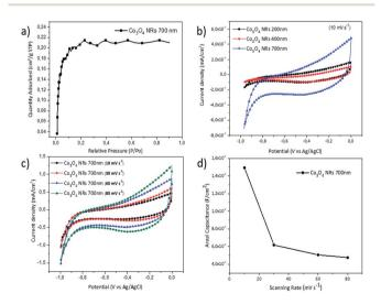
Fig. 6 (a) Isotherm linear plot of N<sub>2</sub> adsorption-desorption of the 700 nm Co<sub>3</sub>O<sub>4</sub> NRs sample. (b) CV curves collected for three different lengths of  $Co_3O_4$  NR electrodes at scan rate of 10 mV s<sup>-1</sup>. (c) Recorded CV data for Co<sub>3</sub>O<sub>4</sub> 700 nm sample with different scanning rates. (d) Variation of areal capacitance versus scanning rate.
