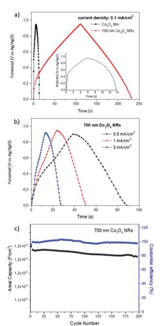
Fig. 7 (a) Charge-discharge profile of 700 nm  ${\rm Co_3O_4}$  NRs and a PVD deposited film (nominal thickness 400 nm). (b) Charge-discharge behavior of 700 nm electrode under different current densities. (c) Cyclic performance for 200 cycles at 0.1 mA cm<sup>-2</sup>.
