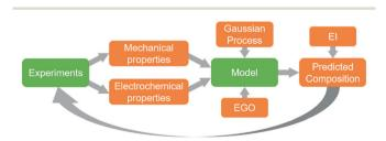
Fig. 3 Schematic showing feedback between the experimental data and the computational model. El is expected improvement and EGO is efficient global optimization.
