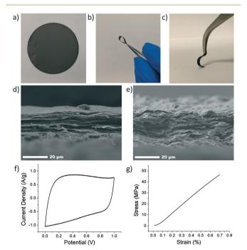
Fig. 4 Digital images of (a) an rGO electrode and (b and c) an rGO/ ANF composite electrode (no CNTs). Cross-sectional SEM images of (d) an rGO/ANF electrode without CNTs (95/5 wt% rGO/ANFs) and (e) with 20 wt% CNTs (76/4/20 wt% rGO/ANFs/CNTs). (f) A representative cyclic voltammogram and (g) a typical stress-strain curve for an rGO/ ANF/CNT composite electrode (90.25 wt% rGO, 4.75 wt% ANFs, 5 wt% CNTs).
