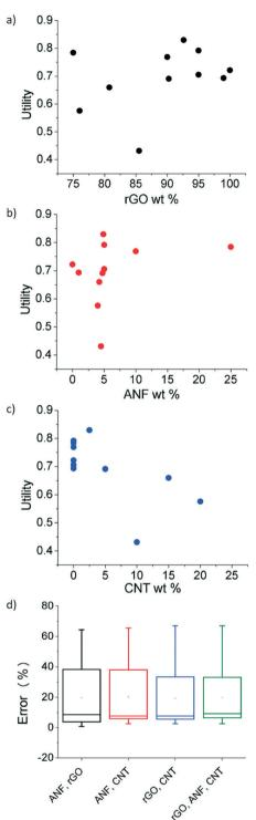
Fig. 5 Utility values for the features (a) GO wt%, (b) ANF wt%, and (c) CNT wt% for each experimental data point. (d) Leave-one-out cross validation error of four different feature sets. Boxes are a statistical representation of the distribution of errors for each feature set. The top and bottom lines are the maximum and minimum data points, the top and bottom of the box are the 75th and 25th percentile markers, the middle line is the median, and the point within the box is the mean.
