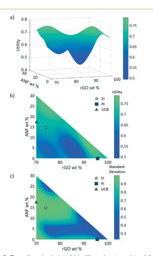
Fig. 6 Three-dimensional plot of (a) utility and contour plots of (b) utility and (c) standard deviation vs. composition. Circular points represent the initial experimental data while the star, square, and triangle represent recommendations from the model based on either expected improvement (EI), probability of improvement (PI), or upper confidence bound (UCB), respectively.
