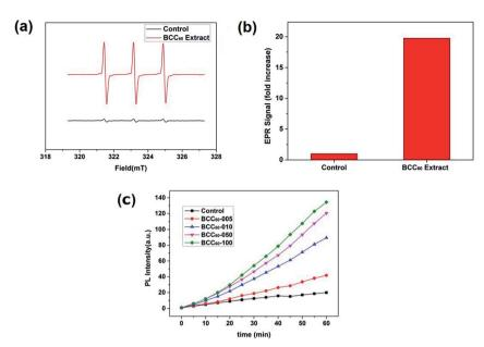
Fig. 4 ROS measurements of the  $BCC_{60}$  composites. (a) and (b) EPR spectra of the  $BCC_{60}$  extract. (c) DCF fluorescence of the  $BCC_{60}$  composites with varying  $C_{60}$  contents after irradiation.
