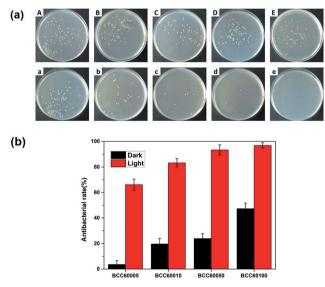
Fig. 5 (a) Antibacterial efficacy of the BC and BCC $_{60}$  composites against *S. aureus* without (A–E) and with (a–e) light irradiation. (A and a) BC, (B and b) BCC $_{60}$ -005, (C and c) BCC $_{60}$ -010, (D and d) BCC $_{60}$ -050, and (E and e) BCC $_{60}$ -100. (b) Antibacterial rate of BCC $_{60}$  against *S. aureus*.
