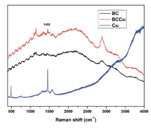
Fig. 2 Raman spectra of the BC, C<sub>60</sub> and BCC<sub>60</sub> composites.
