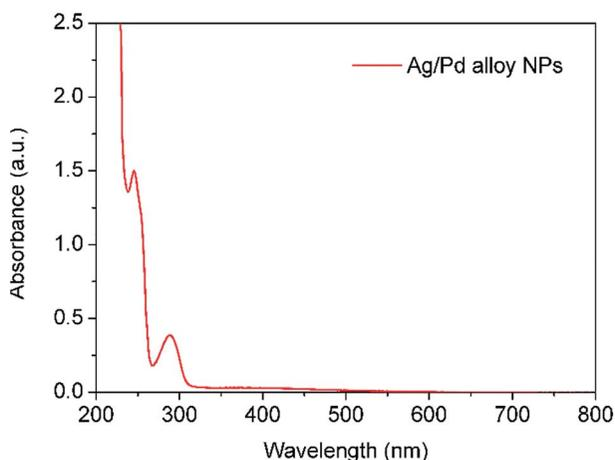
Fig. 12 UV-vis spectrum of Ag–Pd alloy NPs synthesized by simultaneous reduction of  $\text{Ag}(\text{NO}_3)$  and  $\text{Pd}(\text{NO}_3)_2$  with HQ. The solution was diluted for 10 times prior to characterisation.
