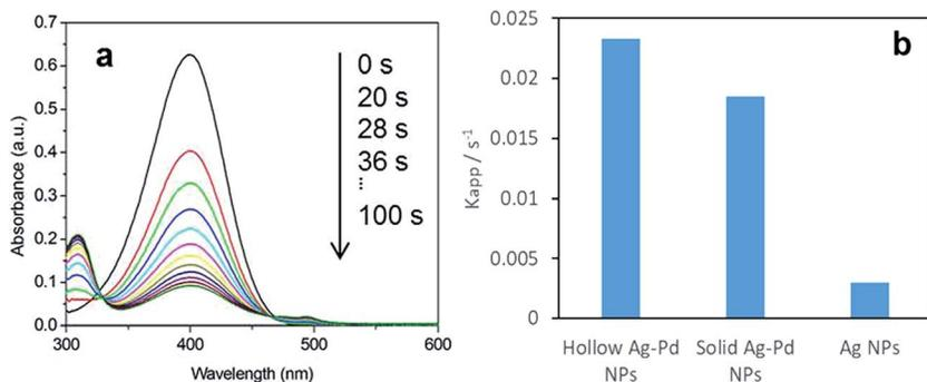
Fig. 16 (a) Time-dependent UV-vis absorption spectra of the catalytic reduction of 4-nitrophenol to 4-aminophenol by an excess amount of  $\text{NaBH}_4$  by hollow Ag-Pd NPs synthesised in 3 CFI reactors connected in series, using  $\text{Pd}(\text{NO}_3)_2$  as precursor. (b) Average kinetic constant ( $K_{\text{app}}$ ) value of hollow alloy Ag-Pd, solid alloy Ag-Pd (synthesised by simultaneous reduction with HQ) and Ag NPs (seeds).
