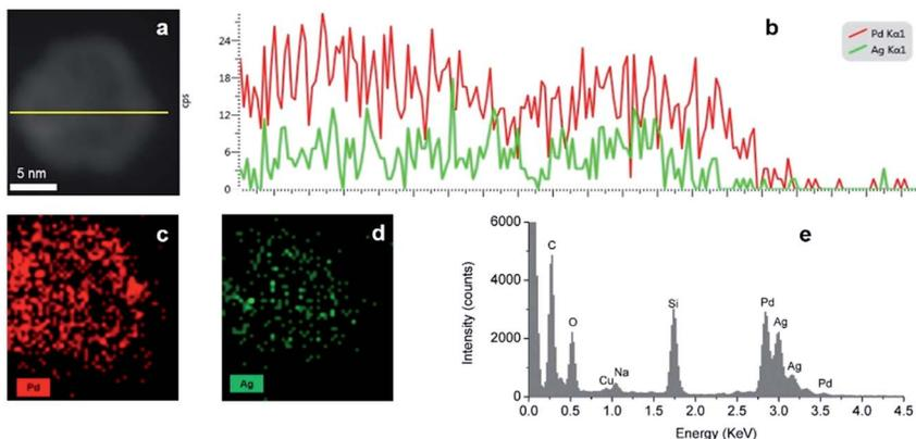
Fig. 7 (a and b) EDS line scan of the Ag–Pd hollow NPs, (c and d) EDS elemental mapping of Ag–Pd hollow NPs, (e) EDS spectra of the Ag–Pd hollow NPs after Reactor 3 using Pd(NO<sub>3</sub>)<sub>2</sub> as precursor.
