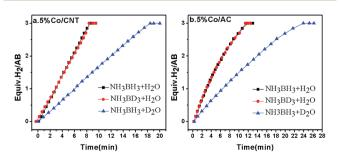
Fig. 1 Hydrogen evolution from NH<sub>3</sub>BH<sub>3</sub> in H<sub>2</sub>O (black), NH<sub>3</sub>BD<sub>3</sub> in H<sub>2</sub>O (red), and NH<sub>3</sub>BH<sub>3</sub> in D<sub>2</sub>O (blue) catalyzed by 5% Co/CNT (left) and 5% Co/AC (right) at room temperature,  $n_{Co}$ :  $n_{AB} = 0.05$ : 1.
