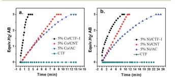
Fig. 3 Plots of volume of H2 generated vs. time for AB hydrolysis catalyzed by (a) 5% Co/CTF-1, 5% Co/CNT, 5% Co/AC, CTF (b) 5% Ni/ CTF-1, 5% Ni/CNT, 5% Ni/AC, CTF. ([AB] = 322 mM, 5 mL,  $n_{\text{metal}}/n_{\text{AB}}$  = 0.05).
