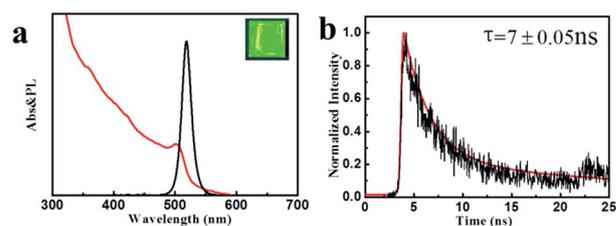
Fig. 3 (a) UV-vis absorption and PL emission spectra (inset: image ( $\lambda_{\text{ex}} = 365$  nm) CsPbX<sub>3</sub> NCs). (b) Time-resolved PL decay and fitting curve for the colloidal CsPbBr<sub>3</sub> NCs sample.
