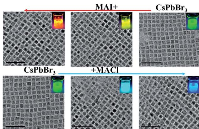
Fig. 4 TEM images of the CsPbBr<sub>3</sub> NCs after treatment with various quantities of MAI (up) and MAI (down). The insets show the evolution of emission colors (under a UV lamp,  $\lambda_{\text{ex}} = 365$  nm) from crude CsPbBr<sub>3</sub> NCs to composited perovskite NCs. Scale bars correspond to 50 nm.
