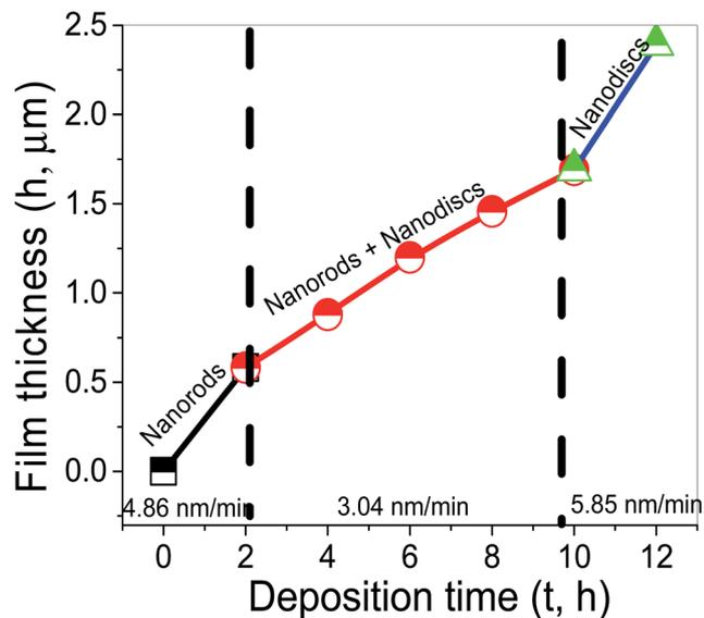
Fig. 7 Variation of film thickness with deposition time.
