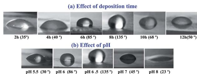
Fig. 15 Contact angles photographs for ZnO nanostructured films fabricated at different (a) deposition time and (b) pH value.
