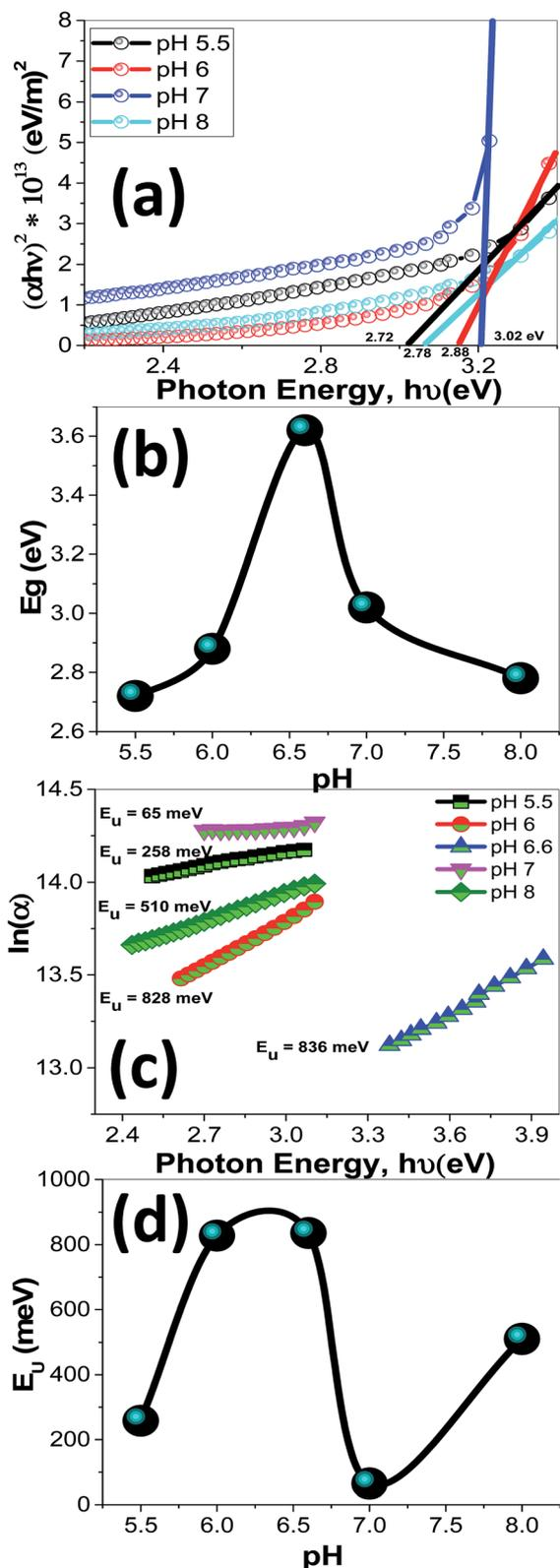
Fig. 14 The plots of (a)  $(\alpha h\nu)^2$  &  $h\nu$  to determine  $E_g$  values, (b)  $E_g$  as a function of pH, (c)  $\ln(\alpha)$  &  $h\nu$  to determine Urbach energy ( $E_U$ ), and (d)  $E_U$  as a function of pH for nanostructured ZnO films.
