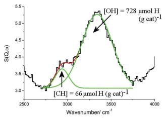
Fig. 16 The INS spectrum  $(2500-4000 \text{ cm}^{-1})$  of a Ni $(45\%)/\text{Al}_2\text{O}_3$  catalyst after undergoing 'dry' reforming of methane at 1073 K for six hours. The experimental data are well described by a combination of two Gaussian curves (green lines) centred at 2935 and 3339 cm<sup>-1</sup>, which are obtained from a non-linear least squares fitting procedure. The solid red line represents the overall fit. Adapted from ref. 78 by permission of the PCCP Owner Societies
