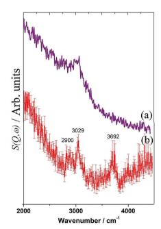
Fig. 17 INS spectra of a Ni(26%)/Al<sub>2</sub>O<sub>3</sub> catalyst after (a) dry reforming and (b) steam reforming of methane at 898 K for six hours.
