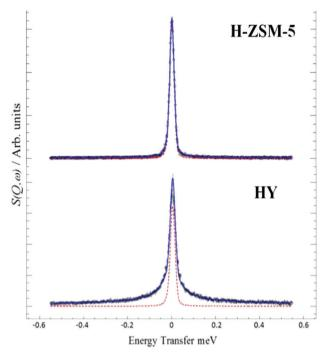
Fig. 13 QENS spectra at 298 K of methanol loaded in zeolites H-ZSM-5 and HY at Q=0.9 Å, (--) represents the resolution data taken at 5 K. Reproduced from ref. 65 with permission of the Royal Society of Chemistry.
