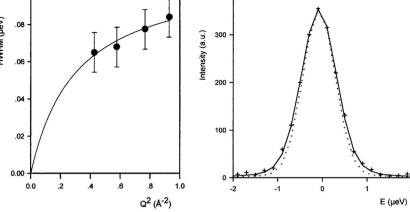
Fig. 6 (left) Broadenings obtained for isobutane in ZSM-5 at 570 K, and QENS spectra obtained at 570 K (Q = 0.87 Å). The dotted line is the resolution function. Reproduced from ref. 55 with permission of the American Chemical Society
