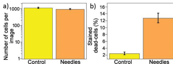
**Fig. 10** Total numbers of (a) bound bacteria and (b) percentage dead cells after 1 h incubation of *P. aeruginosa* on a control ‘flat’ BDD surface and a BDD-coated bSi short-needle surface, and subsequent viability determination by Live/Dead BacLight stain.
