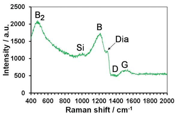
Fig. 3 Raman spectra of the BDD-coated long-needle sample using green (514 nm) excitation. Label key: Dia is the diamond peak, D & G are the disordered and ordered  $sp^2$  carbon bands, respectively, Si is the second-order peak from the bSi substrate, B and  $B_2$  are peaks due to boron and boron-dimer incorporation, respectively.
