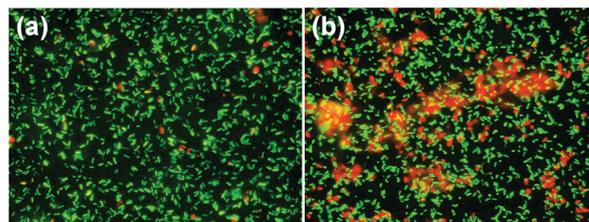
**Fig. 9** Fluorescence micrographs of *P. aeruginosa* after 1 h incubation on (a) a control ‘flat’ BDD sample and (b) a BDD-coated bSi short-needle sample.
