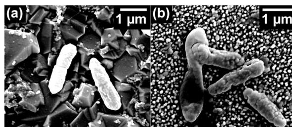
**Fig. 11** Example SEM images of *P. aeruginosa* after 1 h incubation on (a) ‘flat’ BDD surface and (b) BDD-coated short-needle surface. Image (a) shows healthy (turgid) bacterial cells, whereas image (b) shows damaged cells.
