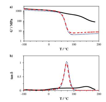
Fig. 3 Storage modulus (G', a) and loss factor ( $\tan \delta$ , b) plots of reference A (—) and mixtures B (+ EAS, ···) and C (+ EVS, ---).
