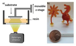
Fig. 5 DLP set up (a) and 3D structures fabricated with formulation C (20 db% EVS, b).
