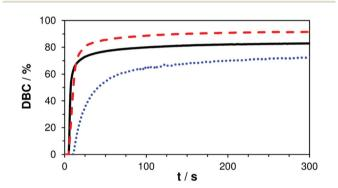
Fig. 2 DBC plots of reference A (—) and mixtures B (+ EAS,  $\cdots$ ) and C (+ EVS, ---); irradiation starts after 5 s.
