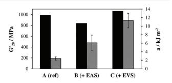
Fig. 4 Storage modulus at 20 °C ( $G'_{20}$ , black) and Dynstat impact resistance (a, grey).
