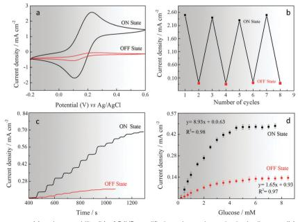
Fig. 3 Cyclic voltammetry response (a) and repeatability (b) of P4VP-modified graphene electrodes in the "on-state" (pH 4) and "off-state" (pH 6). Choronoamperometric response (c) and calibration curve (d) of enzyme immobilised P4VP-modified graphene electrodes in the "on-state" (pH 4) and "off-state" (pH 6) at +0.3 V in 5 mM [Fe(CN)<sub>6</sub>]<sup>3-/4-</sup> and 0.1 M KCl(aq) at 50 mV s<sup>-1</sup> vs. Ag/AgCl reference electrode.
