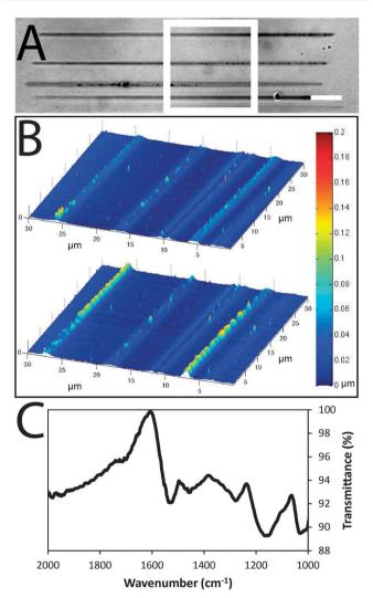
Fig. 2 (A) Optical microscope image of black polypyrrole wires. The dotted white outline represents the scan area for AFM images, and the white scale bar represents 10 µm. (B) AFM image of wires in dry (top) and hydrated (bottom) states. (C) FTIR spectrum of CSA-doped polypyrrole.
