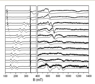
Fig. 2 Single crystal CW X-band EPR of Cr<sub>7</sub>Zn@Ga<sub>7</sub>Zn in the bc plane at 5 K: experimental (thick) and simulated spectra (thin; summation over four molecular orientations, see text). Crystal orientations from  $\theta = 0$  (top) to 90° (bottom); high-field regions  $\times$ 20 for clarity. [The sharp feature at g =1.96 (342 mT) is due to the S = 1/2 excited state.]
