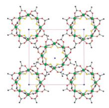
Fig. 1 Unit cell of Cr<sub>7</sub>Zn@Ga<sub>7</sub>Zn viewed down the crystal c axis: Ga/Cr/Zn (green), F (yellow), O (red), N (blue), C (black), Me groups omitted for clarity. See Fig. S1 (ESI†) for full molecule
