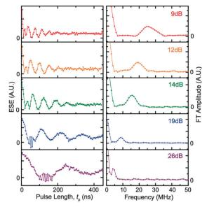
Fig. 4 Left: nutation experiment at 4.5 K measured at  $B_0 = 1160$  mT with  $c \parallel \mathbf{B}$ , for a range of attenuation settings. Right: Fourier transforms of the nutations.
