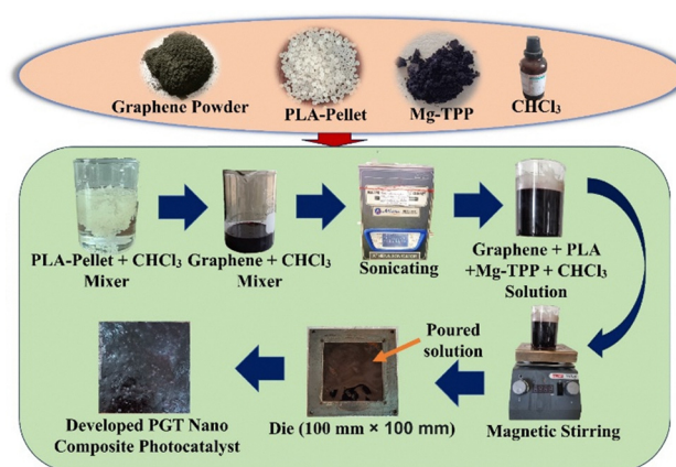
Scheme 4 Synthesis of the PGT nanocomposite flexible artificial leaf photocatalyst.
