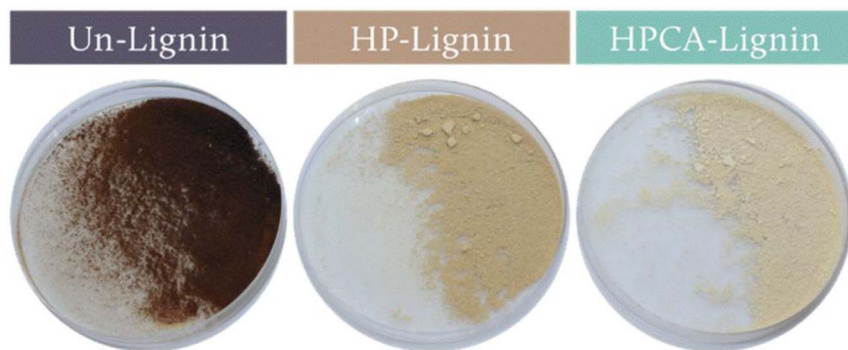
Fig. 7 Visual appearance of bulk unmodified lignin (Un-Lignin), lignin oxidized by the hydrogen peroxide method (HP-Lignin), and lignin oxidized by the peroxy-citric acid method (HPCA-Lignin). Reproduced from Meneses et al. , Faraday Discuss. , 2026, DOI: 10.1039/D5FD00072F with permission from the Royal Society of Chemistry.
