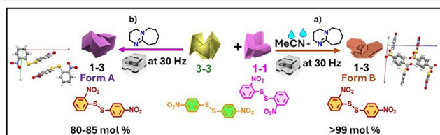
Fig. 14 Effect of milling conditions on the 1-1 + 3-3 disulfide exchange in the presence of DBU. Under NG conditions (left), the reaction yields mostly Form A of 1-3 (80–85 mol%), with 15–20 mol% unreacted 1-1 and 3-3 . Under LAG conditions (right), Form B of 1-3 is obtained quantitatively. 41,53
