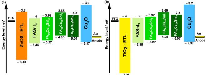
Fig. 6 Band alignment between FASI perovskites with different cesium contents and the ETLs TiO<sub>2</sub> (a) and ZnOS (b). Reproduced from Sabbah et al. (2022),40 (https://doi.org/10.3390/ma15144761). Licensed under CC BY 4.0
