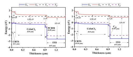
Fig. 10 Band diagrams of PSCs using PCBM and C<sub>60</sub> as ETLs. Reproduced and adapted from Hossain *et al.* (2023)<sup>52</sup> (doi: https://doi.org/10.1038/s41598-023-28506-2) under a Creative Commons Attribution (CC BY 4.0) license.
