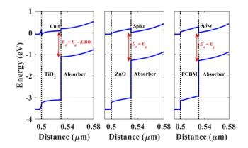
Fig. 5 Band alignment between the perovskite absorber and different ETLs, illustrating cliff and spike profiles. Reproduced from Salem *et al.* (2021)<sup>13</sup> (https://doi.org/10.3390/en14185741). © 2021 by the authors. Licensed under CC BY 4.0.
