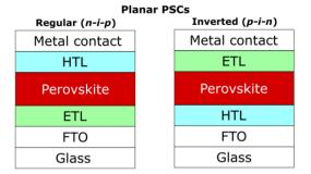
Fig. 1 Regular and inverted planar PSCs.
