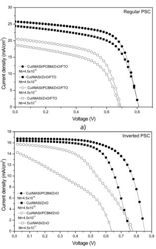
Fig. 8 J-V curves for n-i-p (a) and p-i-n (b) PSCs with and without the use of PCBM as an interlayer, using  $N_t$  values of 4.5  $\times$  10<sup>16</sup> (open symbols) and 4.5  $\times$  10<sup>17</sup> (filled symbols). Reproduced from Araújo *et al.* (2024)<sup>43</sup> (https://doi.org/10.1039/D4RA00634H) under a CC BY 4.0 license.
