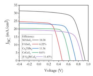
Fig. 9 J-V curves of the PSCs comparing different lead-free perovskites using CZTS as the HTL. Reproduced by Reyes *et al.* (2021)<sup>48</sup> (doi:https://doi.org/10.3390/mi12121508) under a Creative Commons Attribution (CC BY 4.0) license.
