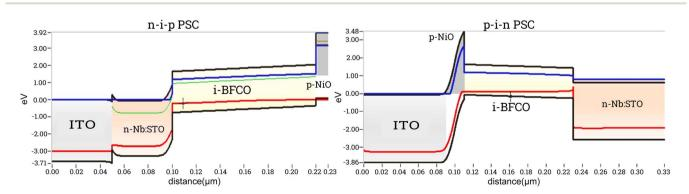
Fig. 15 Band alignment of simulated n-i-p and p-i-n PSCs, reproduced and adapted from Mahammedi et al. (2024)<sup>96</sup> (https://doi.org/10.1016/ j.ijleo.2024.171659) under a Creative Commons Attribution (CC BY 4.0) license.
