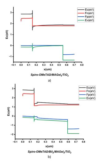
Fig. 13 Energy band alignment of the MAGel<sub>3</sub> perovskite/HTL interface: (a) without and (b) with the Bil<sub>3</sub> interlayer. Reproduced and adapted from Noman *et al.* (2024)<sup>75</sup> (doi: https://doi.org/10.1038/s41598-024-56246-4) under a Creative Commons Attribution (CC BY 4.0) license.
