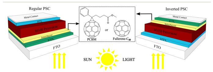
Fig. 7 Fullerene-C<sub>60</sub> and its derivative PCBM used as interlayers in MASI-PSCs with Cul/MASI/ZnO architecture. Reproduced from Araújo et al. (2024)<sup>43</sup> (https://doi.org/10.1039/D4RA00634H) under a CC BY 4.0 license.
