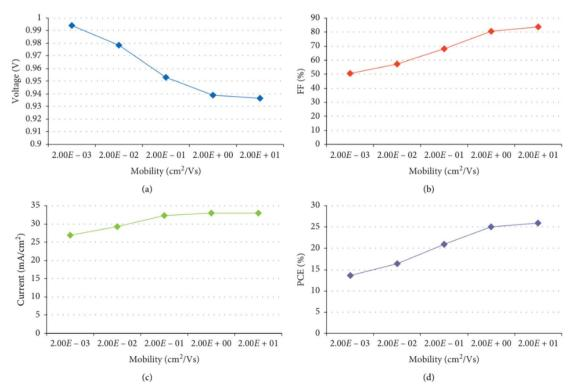
Fig. 12 Variation of  $V_{\rm oc}$  (a), FF (b),  $J_{\rm sc}$  (c) and PCE (d) according to charge mobility, reproduced from Hussain et al. (2021)<sup>70</sup> (https://doi.org/ 10.1155/2021/6668687) under the Creative Commons Attribution License.
