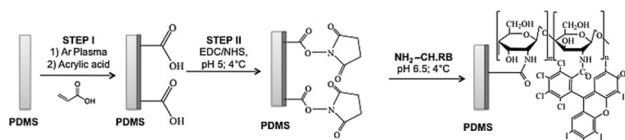
Fig. 4 Schematic illustration of the different steps for PDMS surface modification with CH. RB. Reprinted from ref. 129 Copyright (2013), with permission from Elsevier.
