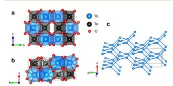
(a) and (b) Monoclinic crystal structure of M-TbTaO<sub>4</sub> (space group Fia. 1 12/a). (c) The distorted diamond lattice of Tb site. The unit cell is shown in thin grey lines.
