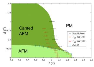
Fig. 9 Proposed magnetic phase diagram for M-TbTaO<sub>4</sub> as a function of magnetic field and temperature. Transition values derived from the magnetic specific heat, magnetic susceptibility ( $T_{N1}$  and  $T_{N2}$ ) and isothermal magnetization are shown as black squares, orange circles, red diamonds, and blue crosses respectively
