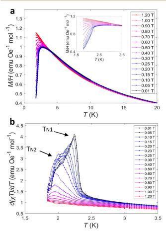
Fig. 3 (a) The ZFC magnetic susceptibility (Inset: At low temperatures) and (b) d( $\chi$ T)/dT ( $\chi \approx M/H$ ) for M-TbTaO<sub>4</sub> as a function of temperature in selected fields.
