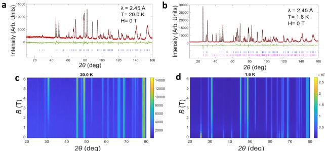
Fig. 6 (a) and (b) Refined PND data of M-TbTaO<sub>4</sub> collected at 20.0 K and 1.6 K respectively with 0 T; (c) and (d) the corresponding heat map showing the evolution of magnetic phase with increasing magnetic field from 0 to 6 T. Red dots, experimental data; black line, calculated intensities; green line, difference pattern; tick marks, nuclear (blue), magnetic (pink) Bragg reflection positions.
