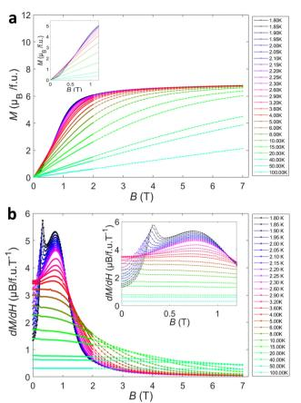
Fig. 4 (a) Isothermal magnetization of M-TbTaO<sub>4</sub> at selected temperatures from 0-7 T (Inset: From 0-1.2 T) and (b) the corresponding derivative, dM/dH as a function of field
