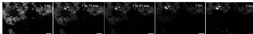
Fig. 5 Ca-K \alpha fluorescence maps extracted from n-XRF spectra at different time points during in situ CaP crystallisation in a liquid cell. Scale bar = 500 nm.
