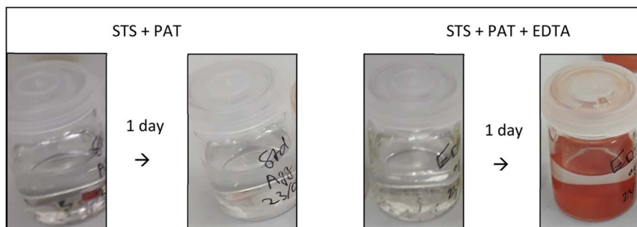
Fig. 4 Vials of \text{Sb}_2\text{S}_3 precursors sodium thiosulfate (STS) and potassium antimony tartrate (PAT) in water (left), and EDTA + STS + PAT in water (right), showing that upon addition of EDTA, a red powder forms over time in ambient conditions. Reproduced from ref. 59 with permission from Royal Society of Chemistry, copyright 2025.
