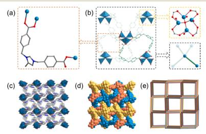
Fig. 1 (a) Coordination mode of the L<sup>-</sup> ligand; (b) [Zn<sub>4</sub>(µ<sub>4</sub>-O)(COO)<sub>4</sub>] secondary building units connected by L<sup>-</sup> ligands; (c) single 3D framework; (d) 3-fold interpenetrated network; and (e) illustration of the 3D topology of the Zn-MOF.
