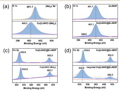
Fig. 3 (a) XPS spectra of N 1s in Cu(i)-NHC-(Me)<sub>2</sub>L and (Me)<sub>2</sub>L<sup>+</sup>Br<sup>-</sup>; (b) N 1s in Zn-MOF and Cu(i)-NHC@Zn-MOF; (c) Cu 2p in Cu(i)-NHC@Zn-MOF and Cu(i)-NHC-(Me)<sub>2</sub>L; (d) Cu 2p in Cu(i)-NHC@Zn-MOF and recycled Cu(i)-NHC@Zn-MOF.
