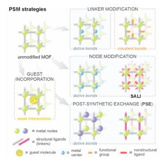
**Fig. 1** Schematic overview and classification of post-synthetic modification (PSM) strategies in MOFs, categorized by the modified framework components and the type of interaction involved (covalent, dative, or noncovalent).
