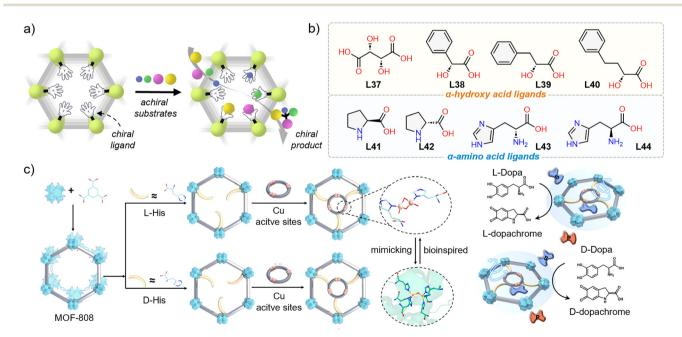
Fig. 6 (a) Scheme of chiral product formation form achiral substrates using CMOF obtained from achiral MOF via SALI method. (b) Examples of  $\alpha$ -hydroxy and  $\alpha$ -amino acid ligands used for SALI. (c) Scheme of two-step functionalization of MOF-808 with L-/D-histidine and Cu(II) ions (left), selective catalytic transformation of L-/b-Dopa to L-/b-dopachrome using L-/b-His-MOF-808 (right). 128 Figure adapted form ref. 128 with permission. Copyright 2023 American Chemical Society
