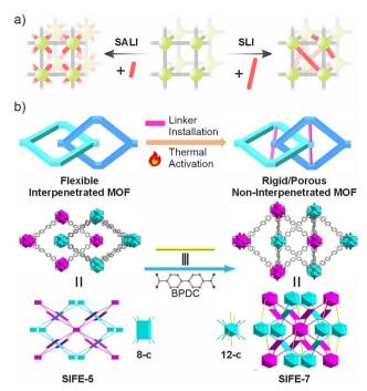
Fig. 11 (a) Scheme of post-synthetic coordination of ligands to inorganic nodes of functionalized MOF showcasing the difference between solventassisted ligand incorporation (SALI) and sequential linker installation (SLI). (b) Installation of rigid struts in interpenetrated flexible MOF leads to its rigidification as exemplified in transformation of SIFE-5 to SIFE-7 material.<sup>200</sup> Figure adapted form ref. 200 with permission. Copyright 2025 John Wiley and Sons.
