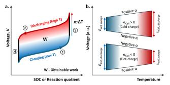
Fig. 1 (a) Voltage-SOC diagram of TREC for  $\alpha_{Cell} > 0$  with its sequence of operation (#1 to #4) and (b) open circuit voltage shifts by electrolyte temperature change for both positive (upper) and negative  $\alpha_{Cell}$  cases (lower).
