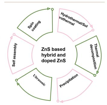
Fig. 2 The different methods of synthesizing ZnS and its heterostructures for CO<sub>2</sub> reduction.
