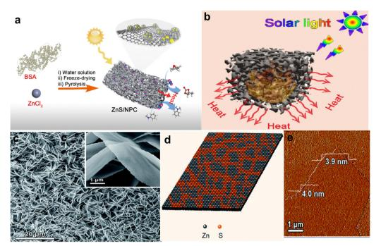
Fig. 5 (a) Schematic illustration of the preparation of ZnS/NPC-X for catalytic conversion of CO<sub>2</sub>, by pyrolyzing protein–Zn( $\parallel$ ) networks. (b) Schematic illustration of the photothermal effect of ZnS/NPC-X (c)-(e) Characterization of S-Zn-S NSs. (c) SEM image; inset shows a typical single nanosheet. (d) Schematic map of the structure of S–Zn–S NSs. (e) AFM image.  $^{73}$
