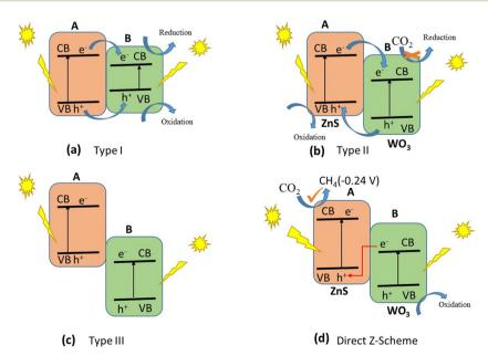
The mechanism of photocatalytic CO<sub>2</sub> reduction on ZnS/WO<sub>3</sub> heterojunctions as they respond to light radiation is depicted schematically
