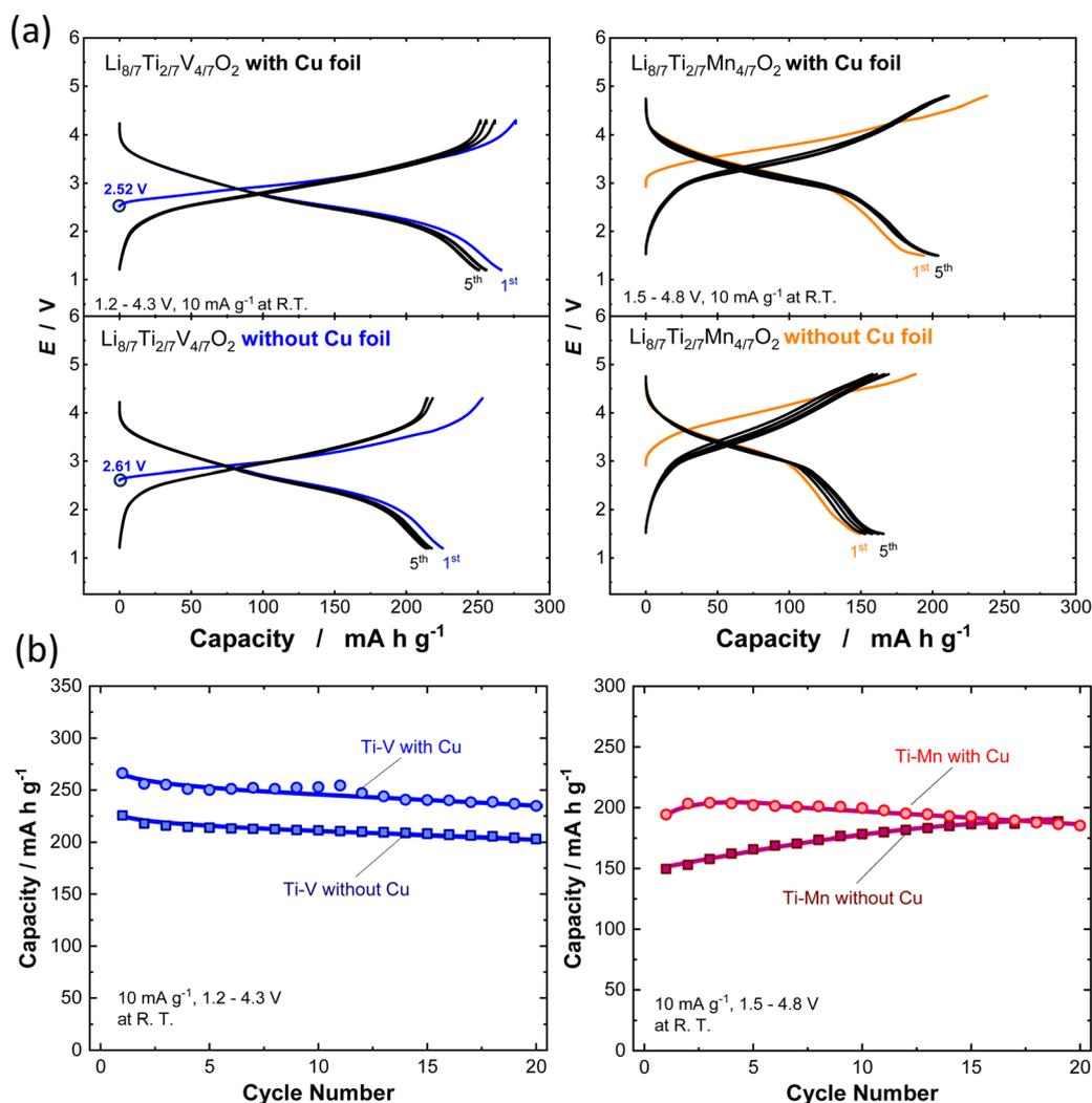
Fig. 3 (a) Galvanostatic charge/discharge curves and (b) discharge capacity retention for 20 cycles of  $\text{Li}_{8/7-x}\text{Ti}_{2/7}\text{V}_{4/7}\text{O}_2$  and  $\text{Li}_{8/7-x}\text{Ti}_{2/7}\text{Mn}_{4/7}\text{O}_2$  synthesized with or without Cu foil at a rate of 10 mA g<sup>-1</sup>.
