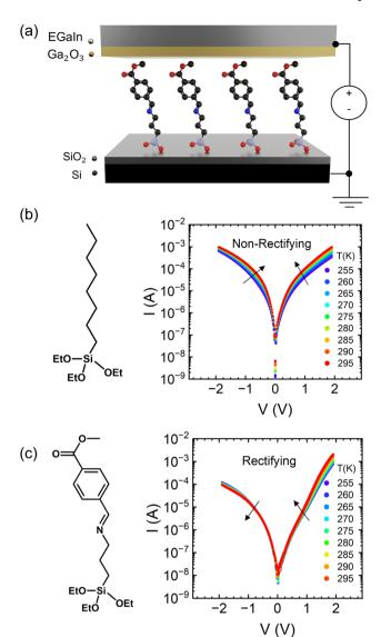
Fig. 1 (a) Device structure of molecular ensemble junctions. (b) Molecular structure and current-voltage characteristics as a function of temperature in the OTES non-rectifying SAM. (c) Molecular structure and current-voltage characteristics as a function of temperature in the CMPTM rectifying SAM.
