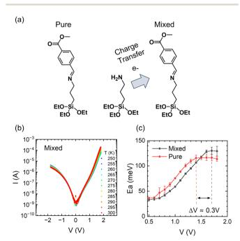
Fig. 4 Schematic of CT occurring between co-assembled CMPTM/ APTES molecules (a). The current-voltage characteristics as a function of temperature for the mixed SAMs of CMPTM:APTES (b) along with the corresponding activation energies (c).
