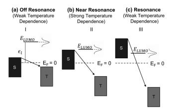
Fig. 3 Energetic landscape of charge transport in a molecular junction governed by eqn (3) when LUMO is the orbital responsible for facilitating transport.  $\varepsilon_1$  represents the energetic position of LUMO, which is placed off resonance in panel (a), near resonance in (b), and in resonance (c)
