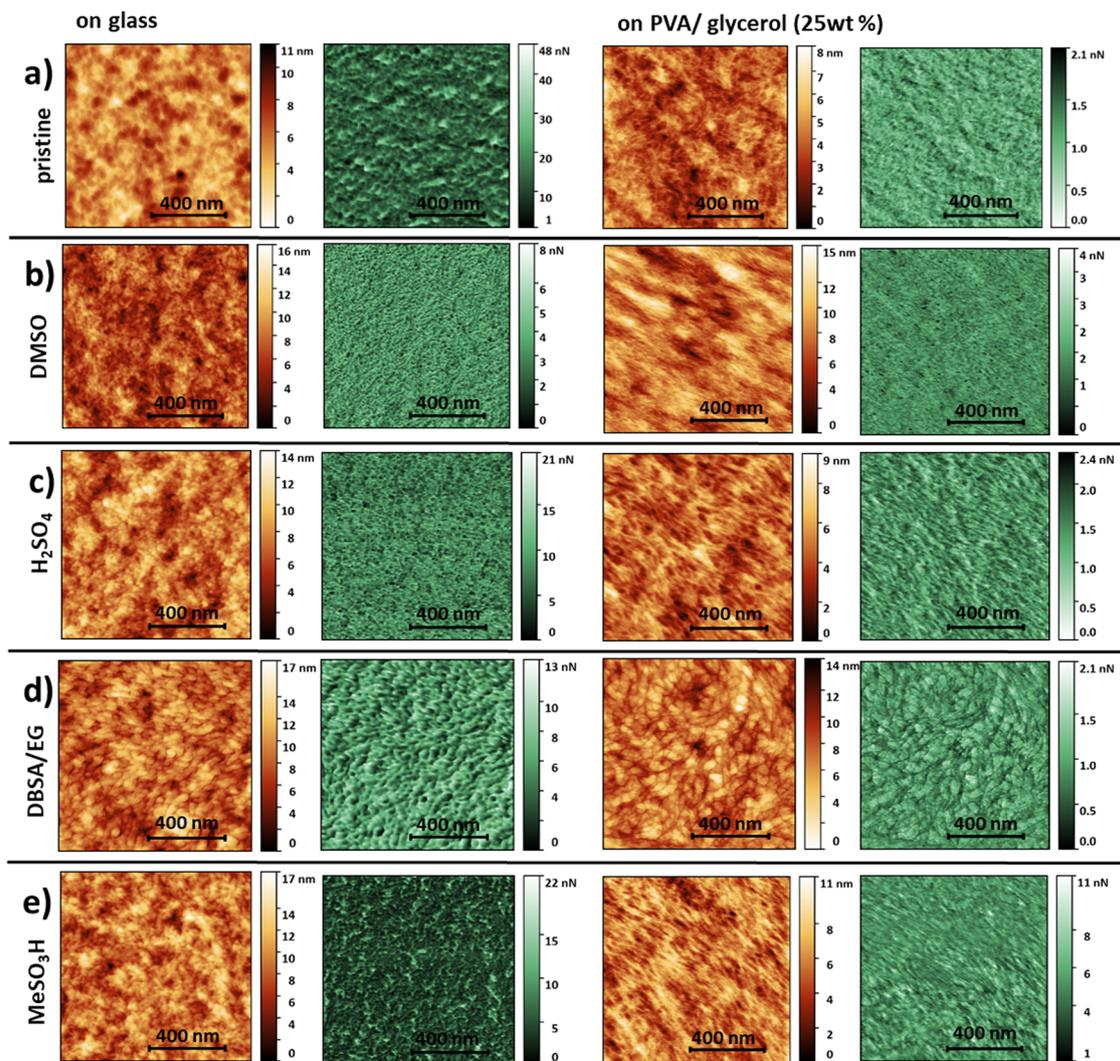
Fig. 2 SFM images recorded in Peak Force mode. We selected an orange color scale for topography and a green color scale for the corresponding adhesion forces. (a) pristine (PH1000), (b) DMSO<sup>12-</sup>, (c) H<sub>2</sub>SO<sub>4</sub><sup>2-</sup>, (d) DBSA/EG<sup>37-</sup> and (e) MeSO<sub>3</sub>H<sup>2-</sup>-treated PEDOT:PSS thin films on glass (left) and transfer-printed onto PVA/Glycerol (25 wt%), right. All scale bars correspond to 400 nm.
